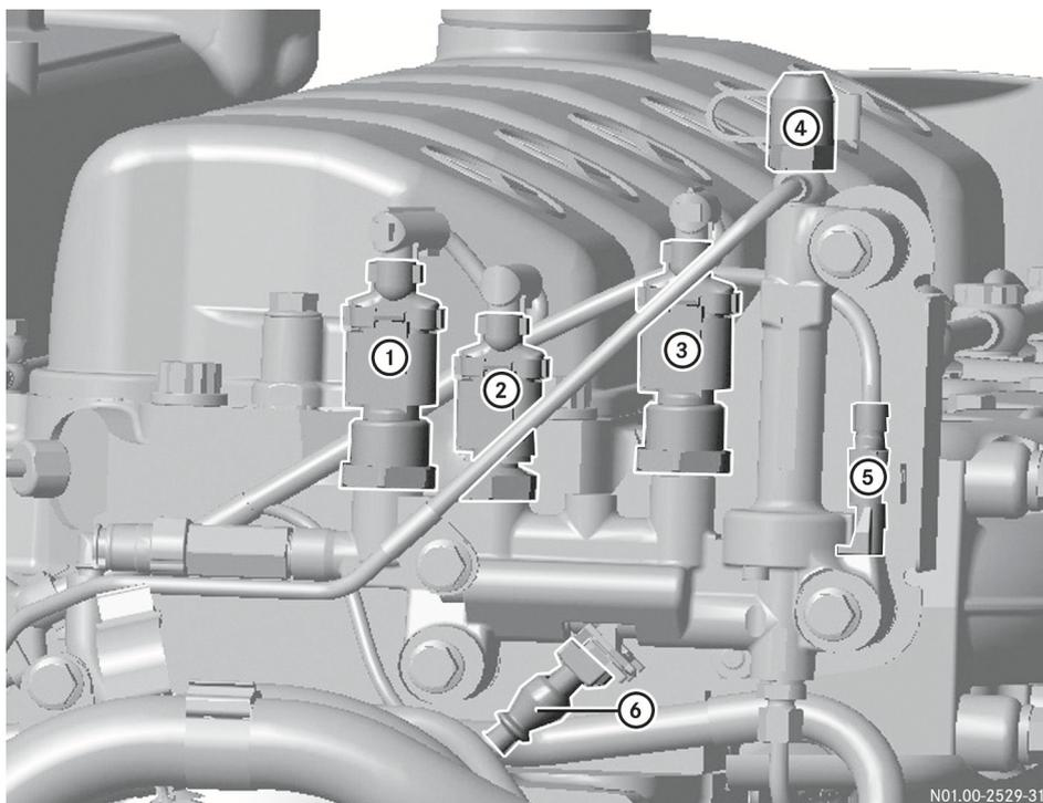
BlueTec® sensors and test connection on the metering unit
