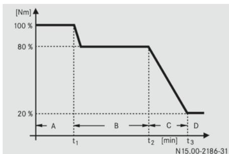
Poor AdBlue®/DEF quality and misuse; warning and length of operating restriction period (example display)
