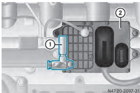
Fuel system on crankcase (left side of engine)
