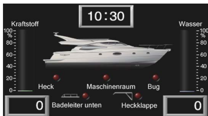
Figure: start page with fuel tank levels, bilge status and door monitoring
